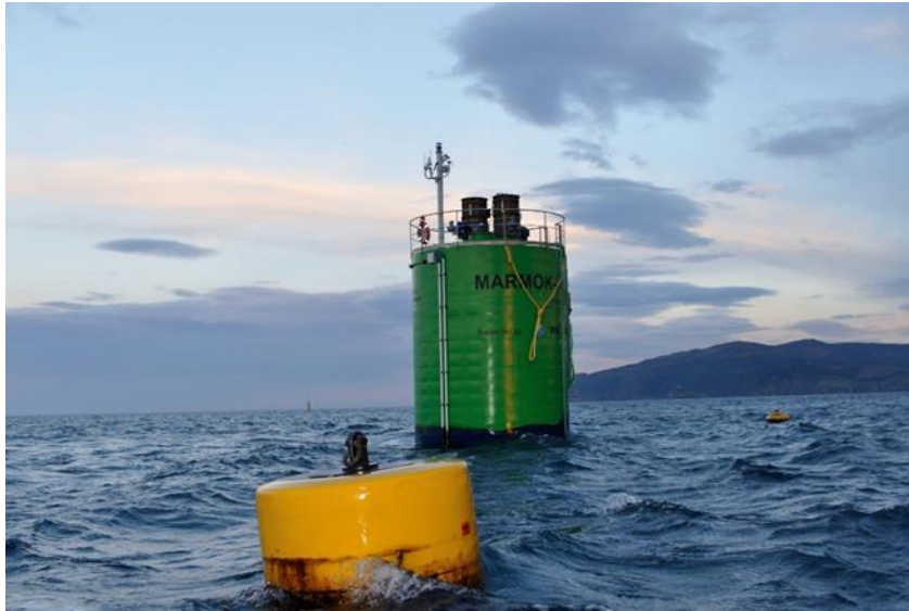
FIGURE 2-1 MARMOK-A-5 DEVICE DEPLOYED IN BIMEP
