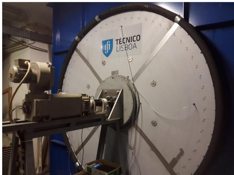
**FIGURE 2: EXPERIMENTAL SETUP, SHOWING THE ELECTRICAL GENERATOR, THE HORIZONTAL-AXIS TURBINE AND THE PLENUM CHAMBER. THE DIFFUSER IS LOCATED INSIDE THE PLENUM CHAMBER.**
