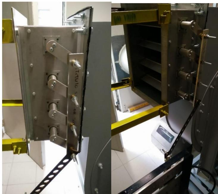
**FIGURE 19: VARIABLE AIR-FLOW VALVE.**
